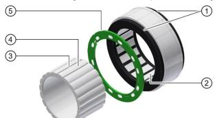
**The Stator** consists of a steel core made of bonded laminations with the copper motor windings (2) and a circuit board (5) with an NTC-thermistor and the connections for the windings on an isolating plastic carrier (1).
