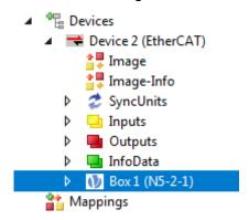
6 By clicking on **Box 1** and selecting the Tab **CoE-Online** you can see the object-dictionary of the drive and could add startup-values if needed.
